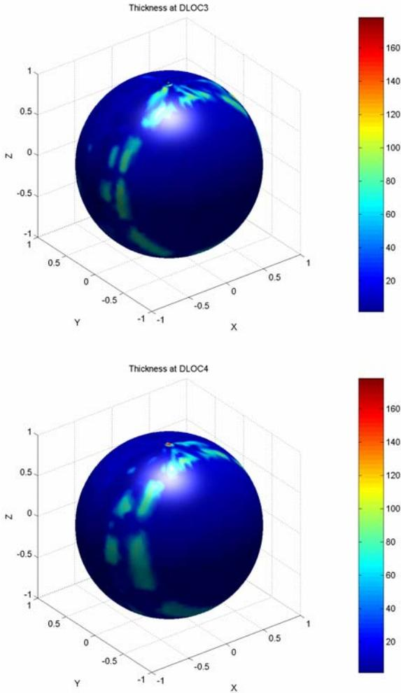
Figure 3b. Shielding distributions at the other 2 locations inside a spacecraft: DLOC3 and DLOC4.
