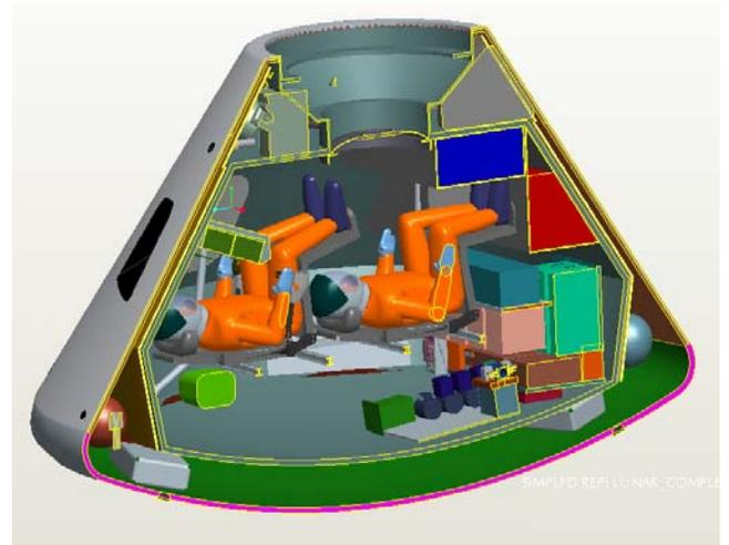
Figure 2. Structural distribution model of various composition layers for exploratory-class spacecraft developed using ProE™
