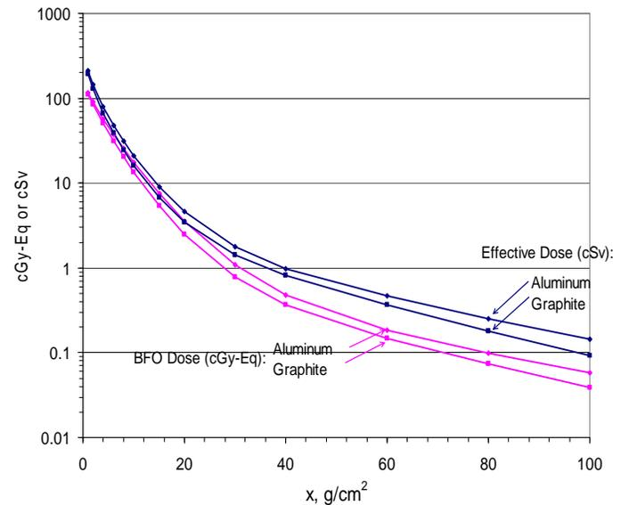
Figure 1. Effective dose and BFO dose behind aluminum and graphite shielding materials in free space from August 1972 solar particle event.
