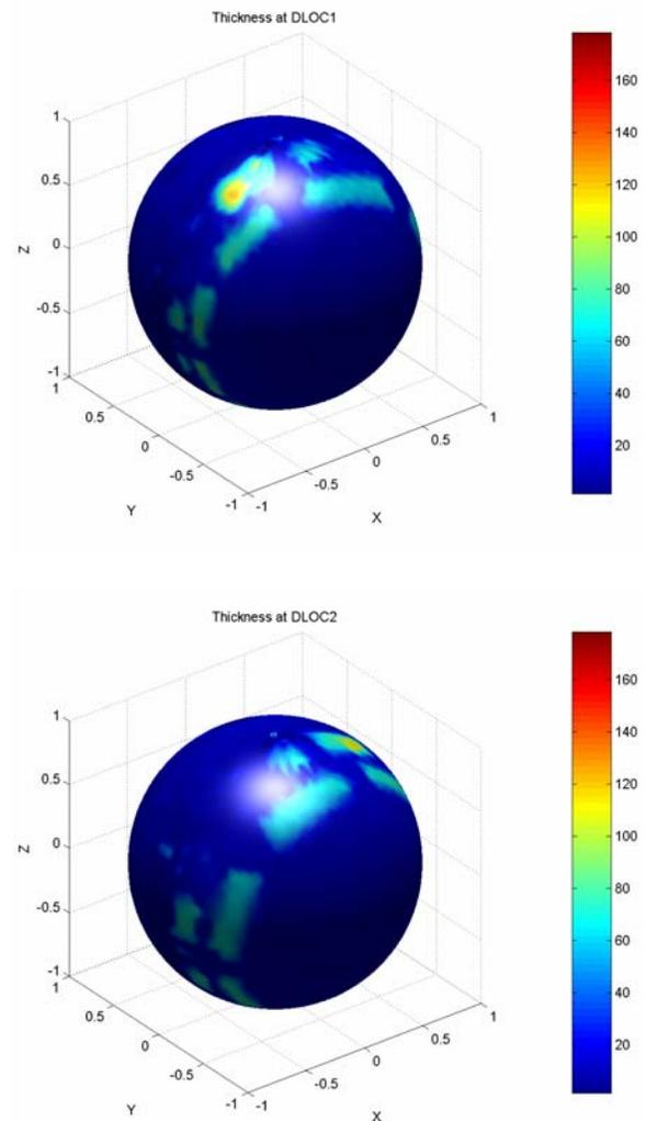
Figure 3a. Shielding distributions at 2 locations inside a spacecraft: DLOC1 and DLOC2.
