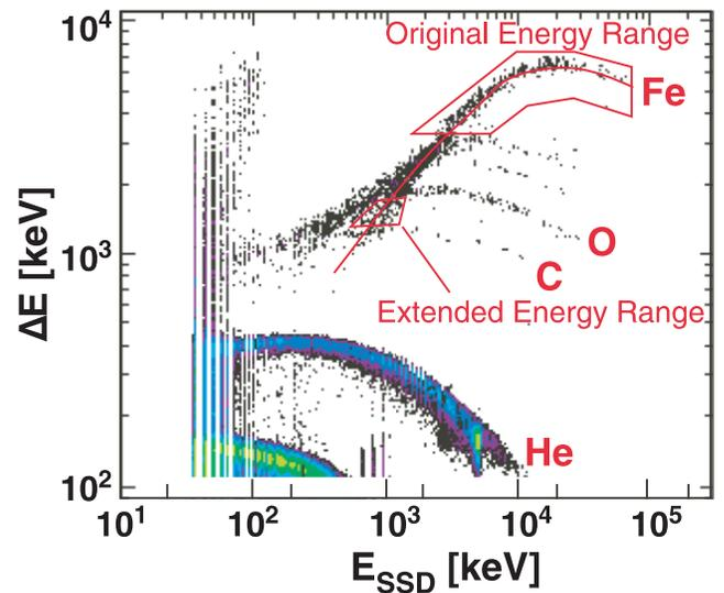
FIG. 1.—Energy loss ( $\Delta E$ ) in the proportional counter vs. energy ( $E_{SSD}$ ) measured in the SSD. Each ion species leaves a unique track. At energies below 0.18 MeV nucleon<sup>-1</sup> the tracks for different ion species start to merge. However, the Fe track crosses over the O track and then re-emerges with only small interference from N. Red labeled boxes show the original Fe energy range and the extended range introduced in this work.
