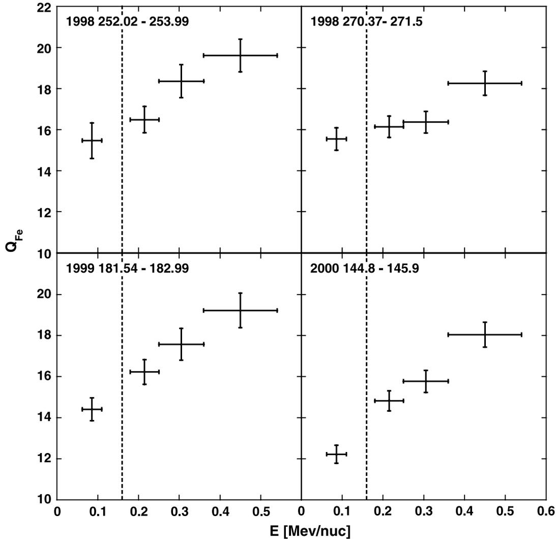
FIG. 2.—Fe charge states vs. energy (both linear) for four different impulsive events with good counting statistics. The error bars along the energy axis indicate the individual energy ranges, and the ones along the vertical axis show the statistical uncertainty of the mean charge states. The data point to the left of the dashed line has been taken from the extended energy range.
