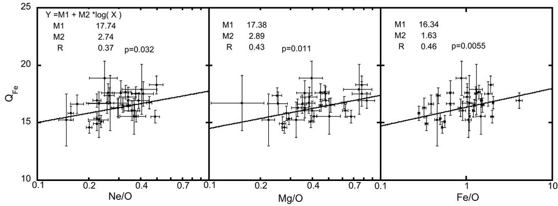
FIG. 4.—Fe charge states in the energy range 0.18–0.43 MeV nucleon<sup>-1</sup> (linear) as a function of heavy ion abundance ratios at the center energy of 0.24 MeV nucleon<sup>-1</sup> from *ACE* ULEIS (logarithmic). *Left*: Ne/O; *middle*: Mg/O; *right*: Fe/O. A logarithmic fit has been applied to each data set whose fit lines and parameters are included.
