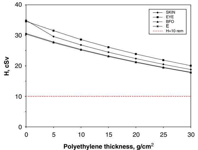
Fig. 5. Dose equivalents at sensitive sites with various polyethylene shields inside 20 g/cm<sup>2</sup> of aluminum from February 23, 1956 SPE.
