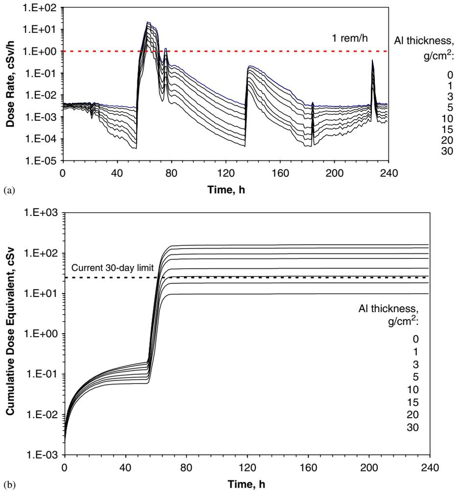
Fig. 3. (a) BFO dose rate during August 2–11, 1972 SPE; (b) Cumulative BFO dose equivalent during August 2–11, 1972 SPE.
