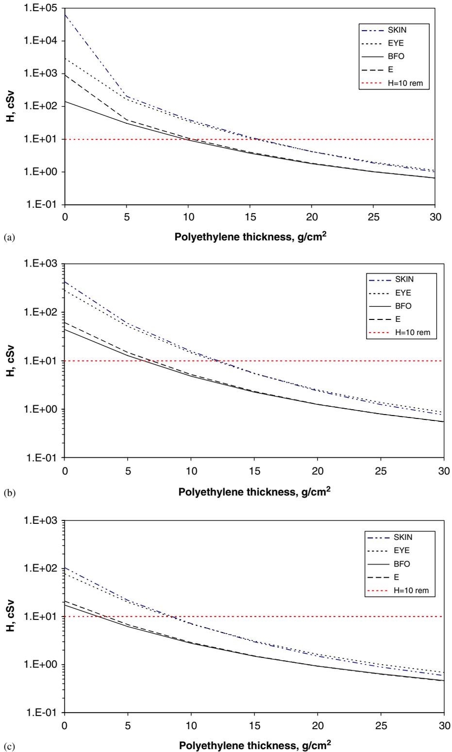
Fig. 6. Dose equivalents at sensitive sites from August 1972 SPE with various polyethylene shielding inside (a) 0; (b) 5, and (c) 10 g/cm<sup>2</sup> of aluminum.
