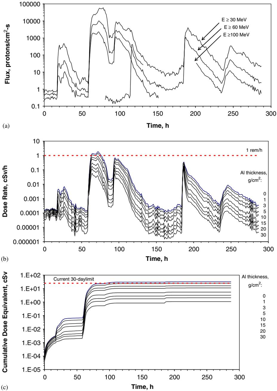
Fig. 2. (a) Hourly averaged proton flux during October 26–November 6, 2003 SPE; (b) BFO dose rate during October 26–November 6, 2003 SPE; (c) cumulative BFO dose equivalent during October 26–November 6, 2003 SPE.
