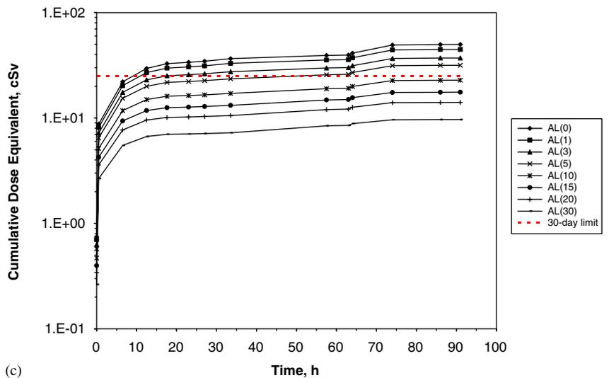
Fig. 4. (a) Proton flux at time of measurement during November 12–16, 1960 SPE; (b) BFO dose rate during November 12–16, 1960 SPE; (c) cumulative BFO dose equivalent during November 12–16, 1960 SPE.
