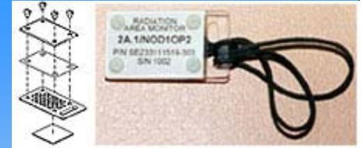
The Radiation Area Monitor (RAM) is a small set of thermoluminescent detectors (TLD) encased in a Lexan holder
