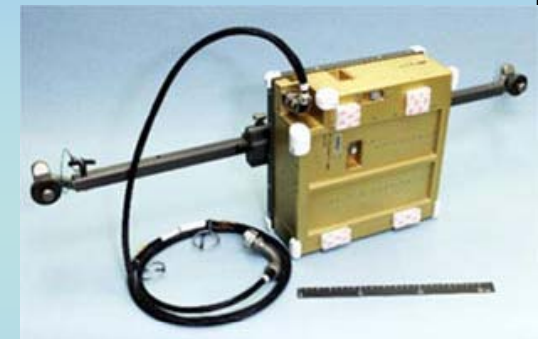
The IV-CPDS displays the average dose rate and other parameters on a small LCD screen on the instrument for use by the astronauts, and sends similar information to Mission Control
