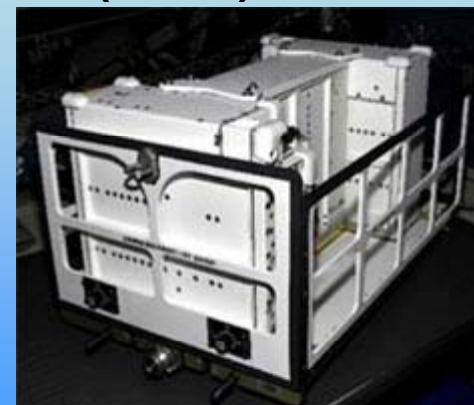
EV-CPDS: three CPDS instruments are mounted outside the ISS
